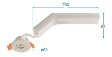
**Specification:** Stand-alone self-contained emergency LED downlight. Constant emergency light (1.5W/150Im & 3W/270Im) for 3 hours. Low stand-by power consumption (0.5W). Self-test versions and remote controls available. Lithium battery integrated. Non-maintained configuration. Ceiling recessed mounting. Suitable for open area and corridor indoor applications.
