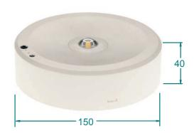
Specification: Stand-alone self-contained emergency LED downlight. Open area lens integrated. Constant emergency light (1.5W/150lm) for 3 hours. Low stand-by power consumption (0.5W). Self-test versions and remote controls available. Lithium battery integrated. Non-maintained configuration. Ceiling surface mount. Suitable for open area and corridor indoor applications.
