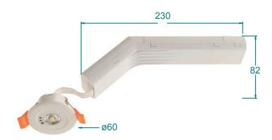
**Specification:** Stand-alone self-contained emergency LED downlight. Open area lens integrated. Constant emergency light (3W/270lm) for 3 hours. Low stand-by power consumption (0.5W). Self-test versions and remote controls available. Lithium battery integrated. Non-maintained configuration. Ceiling recessed mounting. Suitable for open area and corridor indoor applications.
