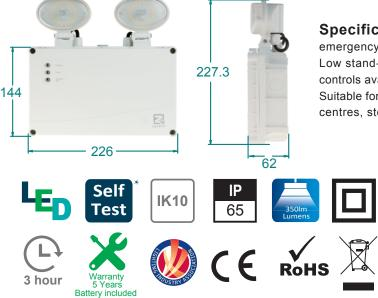
**Specification:** Weatherproof (IP65) and robust (IK10) self-contained emergency LED twin spot. Constant emergency light (350lm) for 3 hours. Low stand-by power consumption (0.5W). Self-test versions and remote controls available. Lithium battery integrated. Non-maintained configuration. Suitable for indoor and outdoor applications such as car parks, distributions centres, storage rooms, warehouses and large open space areas.
