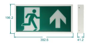
**Specification:** Slim self-contained emergency LED exit sign box. Viewing distance 34m. Constant emergency light (70lm) for 3 hours. Low stand-by power consumption. Self-test versions and remote controls available. Lithium battery integrated. Maintained or non-maintained configurations. Suitable for indoor applications such as educational and offices buildings.
