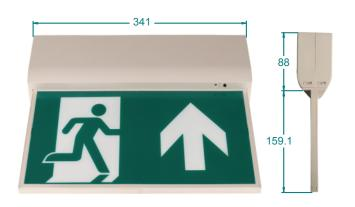
**Specification:** Double sided self-contained emergency LED exit sign. Viewing distance 30m. Constant emergency light for 3 hours. Low stand-by power consumption. Self-test versions and remote controls available. Lithium battery integrated. Maintained or non-maintained configurations. Ceiling or recessed mounts. Suitable for indoor applications such as educational and office buildings.
